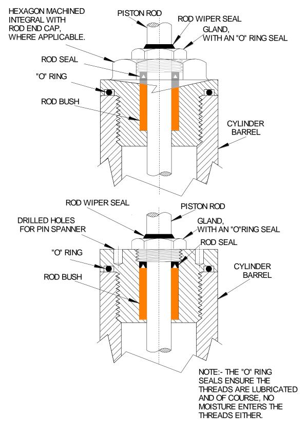
IT IS IMPORTANT TO NOTE THAT THE ROD SEAL IS POSITIONED SO THAT THE ROD BUSH IS LUBRICATED WITH THE HYDRAULIC FLUID.
