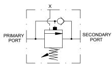
OVERCENTRE VALVE OR BRAKING VALVE. PORT X = REMOTE PILOT SIGNAL PORT.
