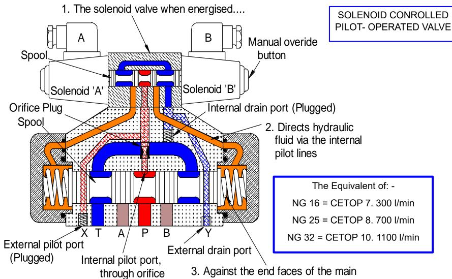
4. Via Port "P" to either Port "A" or "B" spool to direct the pump flow rate.... to the actuator (Cylinder or Hydraulic motor)
