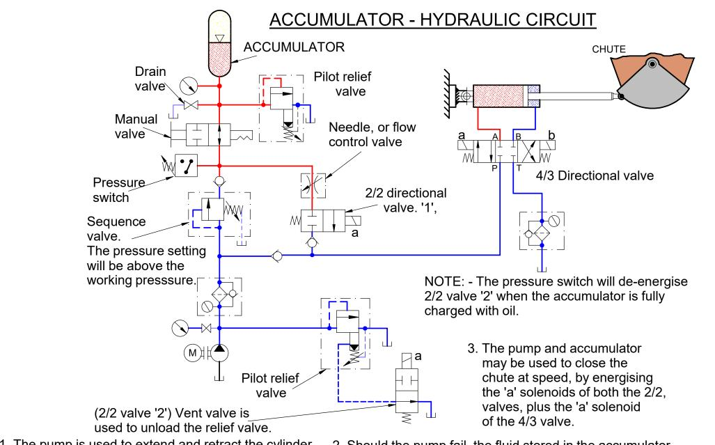
1. The pump is used to extend and retract the cylinder, to open and close the chute, by energising the 'a' solenoids of the 2/2 vent valve '2', and the 'a' or 'b solenoid of the 4/3 valve.
